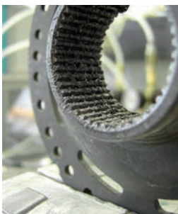
Interior spray greasing
