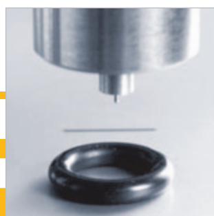
Tensile strength test (left picture) and hardness tests of elastomers
